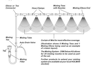
Work out the spacing of the misting jets and cut the misting hose to length and install the relevant misting tees. Finish each line with a misting elbow.
